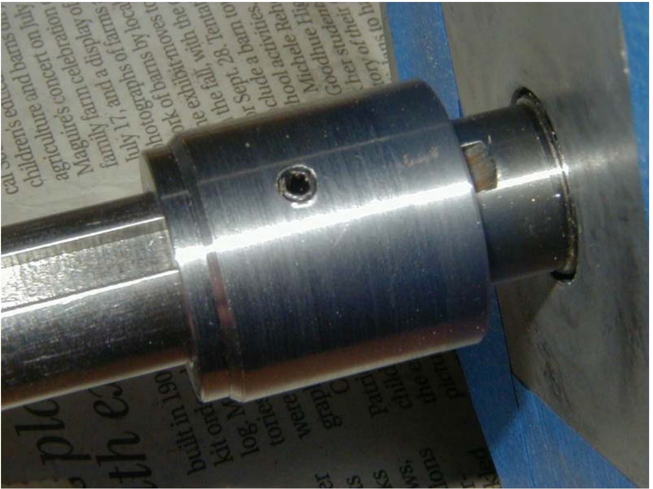
The pin has been inserted through the collar and motor shaft.
