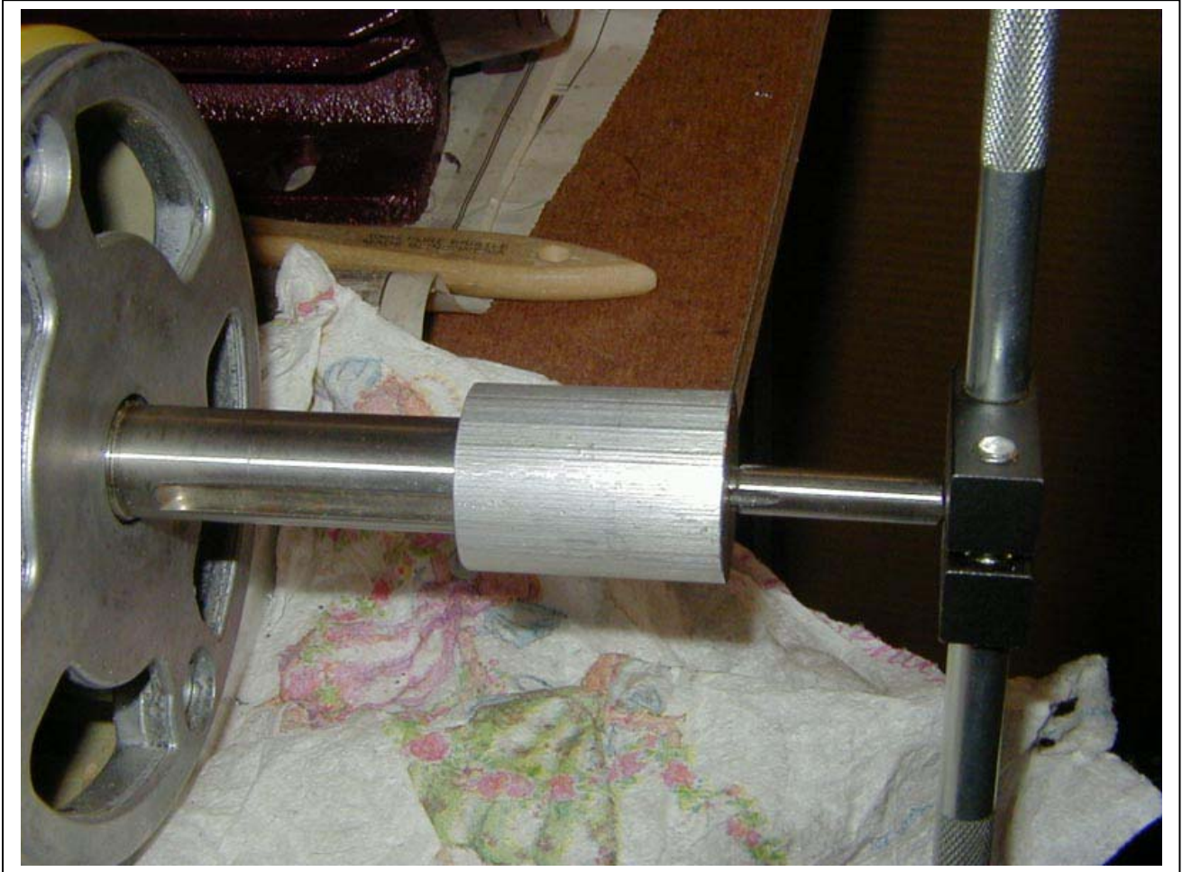
This picture shows the drill/tap guide in use tapping the hole in the motor shaft.
